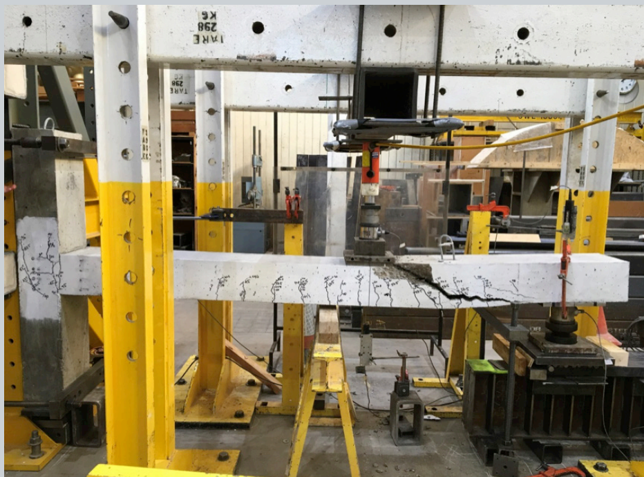
Figure 1 - Test arrangement and failure mode in shear
